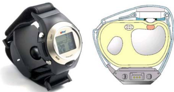
Figure 2: The BPro™ watch showing the tonometer integrated into the watch strap. The diagram shows the tonometer positioned over the radial artery when the watch is worn for recording ambulatory radial wave-forms calibrated to brachial pressure.
